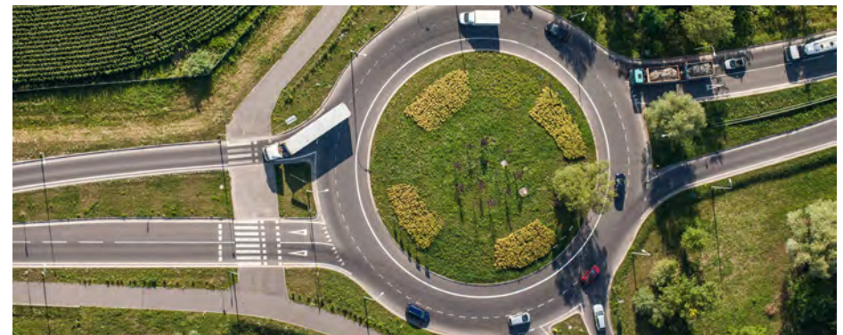
FIGURE 4. EXAMPLE OF A ROUNDABOUT
